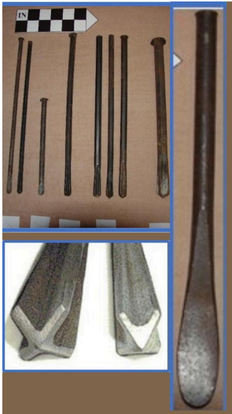
Top left – start drills and deep hole mud spoon (Courtesy of Mary Gage and James Gage, www.stonestructures.org ); top right – deep hole mud spoon; bottom left – star drill tip. (Photos: PSK)
